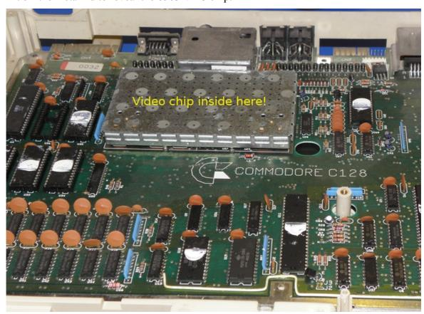
3. Carefully remove the 8563 VDC chip from it's socket.
