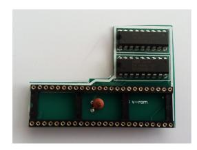
The VDC (Video Display Controller) RAM Upgrade Module is a solder-less, easy to install, video memory upgrade for the Commodore 128 and 128D. The standard C128 and C128D has just 16K of video RAM, this upgrade gives you a full 64K, like the C128DCR.
